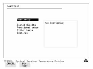
With Smartsetup highlighted, press **RUN TEST** to auto-discover information about the receive signal. Or press **CANCEL** to exit Smart Tests.
