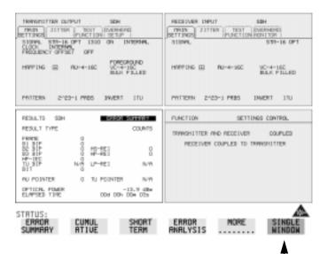
Press this key to select single window mode. The active window is then displayed (in this example - RESULTS would be displayed).
